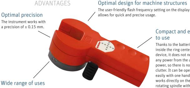
The open design can be placed over the spindle from the side, meaning there is no obstruction from the thread guide or balloon control ring. The ring traveler can remain on the centering ring. Ring Range 36 mm to 54 mm. Spindle diameters of 16 mm to 18 mm.
