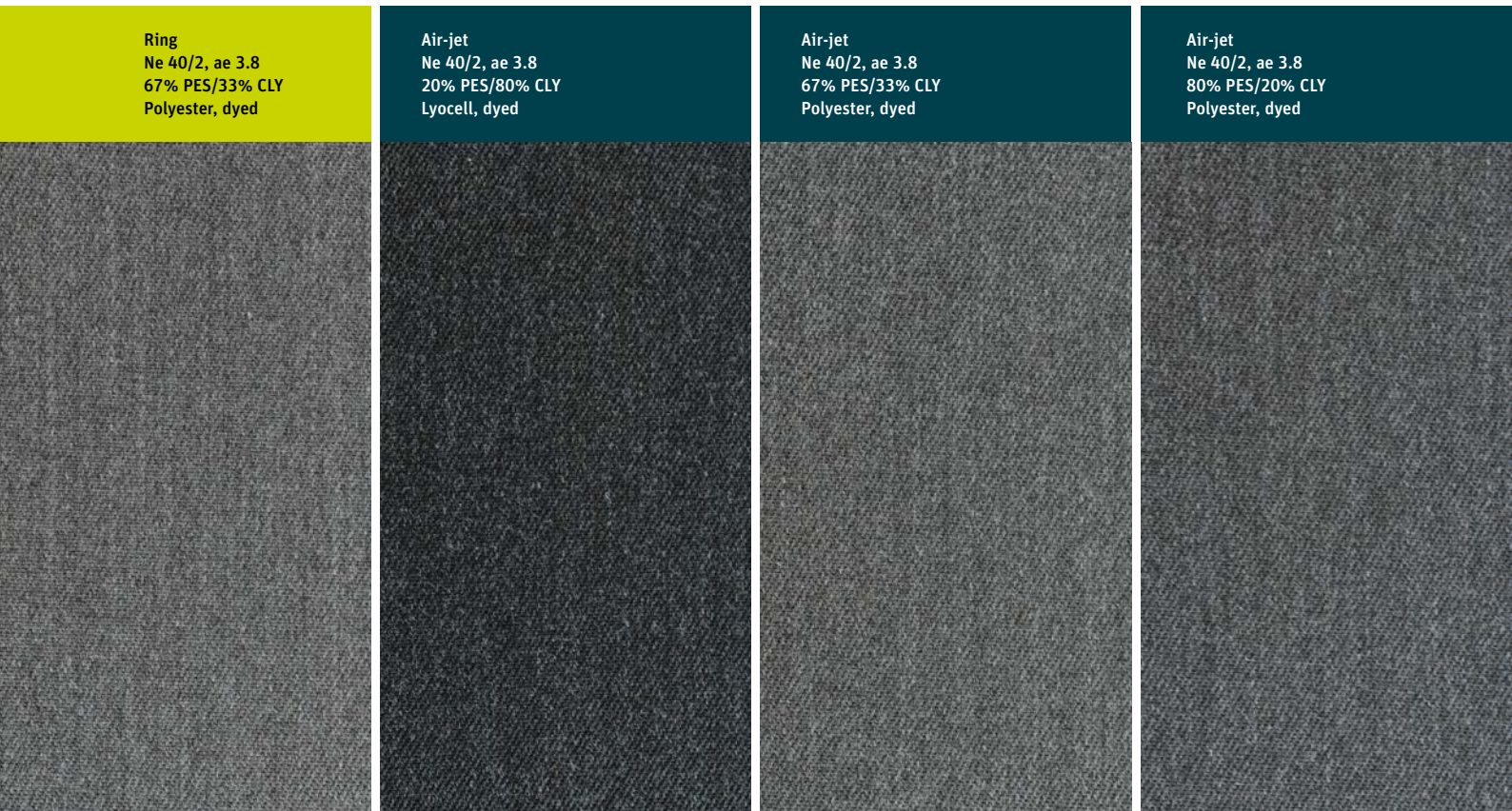
Fig. 8: The woven fabrics produced from various polyester/lyocell blends demonstrate the desired wool effect.
