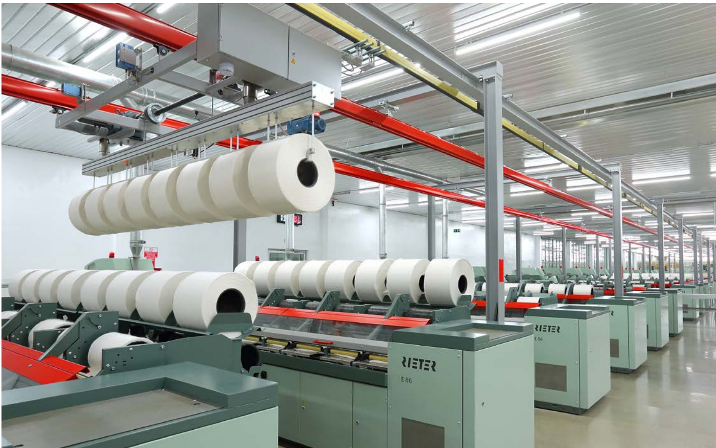
Fig. 1: The E 26 is efficient at transporting laps from the OMEGAlap E 36 to the combers, and takes up little space.
