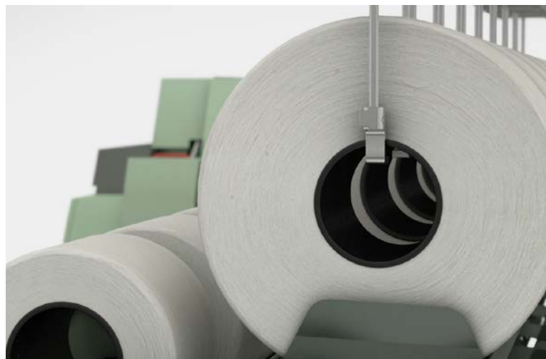
Fig. 3: Quality is ensured, since the batt remains untouched during the entire lap transport process.
