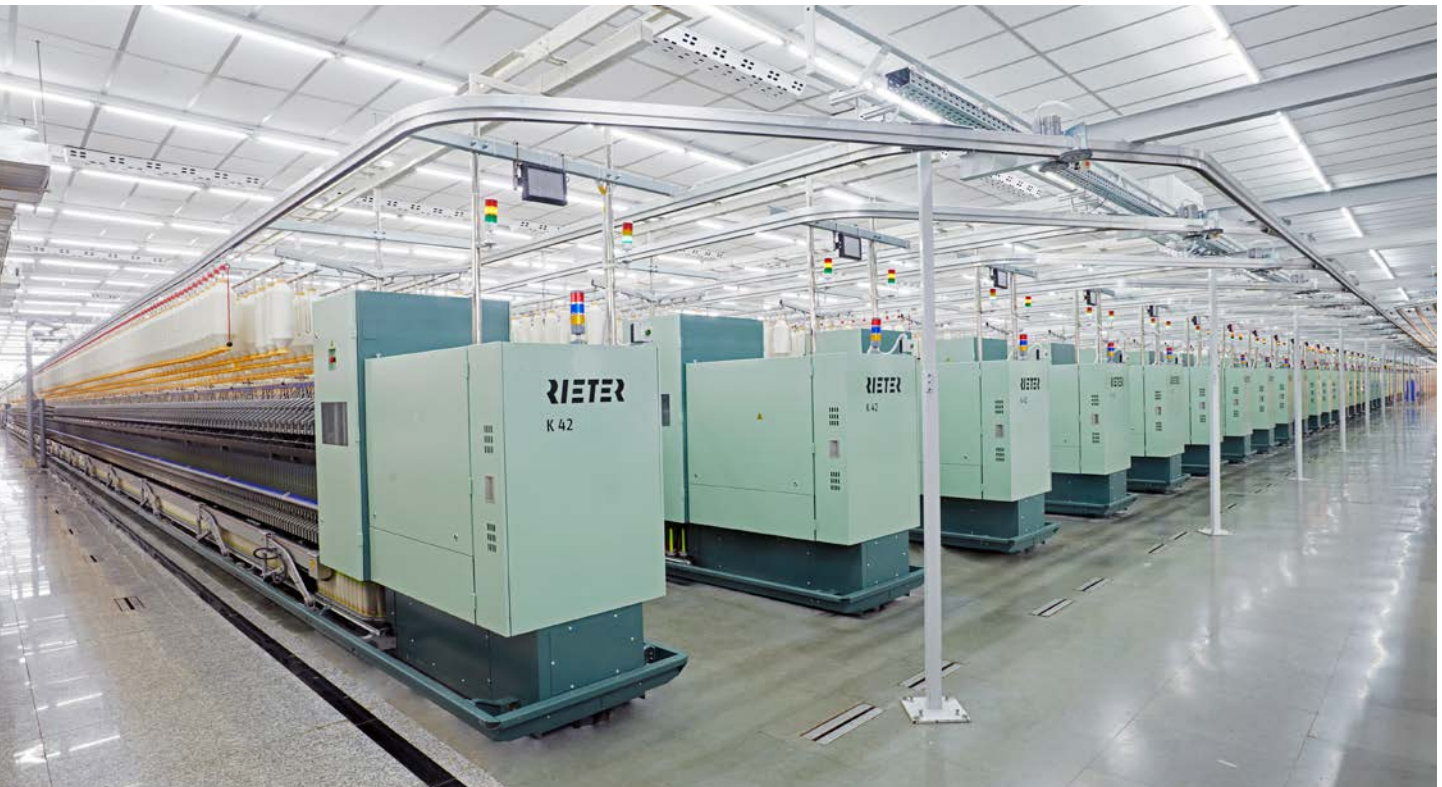
Fig. 1: High yarn quality thanks to the compact spinning machine K 42
