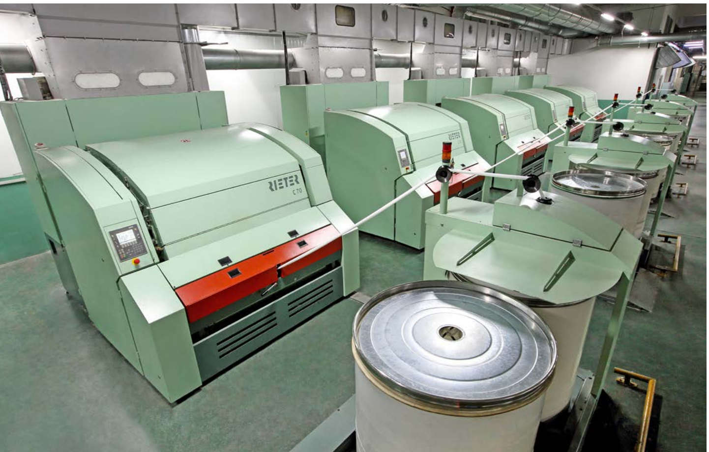
Fig. 1: The card C 70 produces card sliver with excellent quality values.
