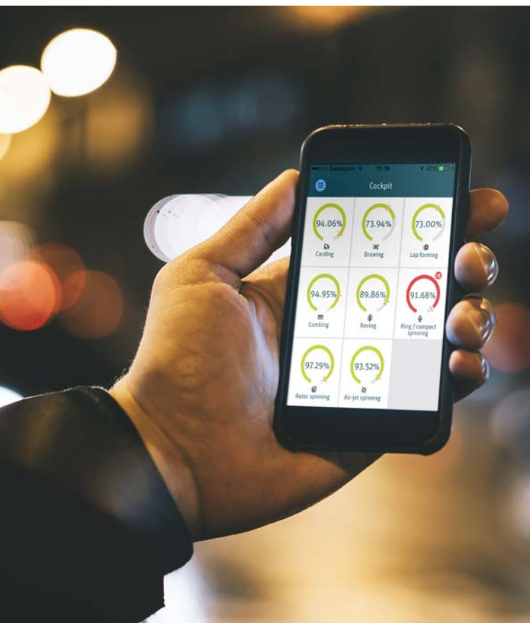
Fig. 1: The cockpit function provides a production overview of spinning machines from anywhere at any time. This allows a quick response and prevents costly downtimes.
