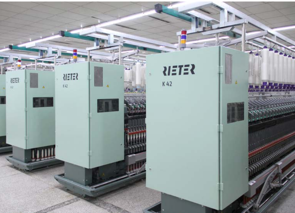
Fig. 1: The compact-spinning machine K 42 can achieve better results than those currently being achieved in China.
