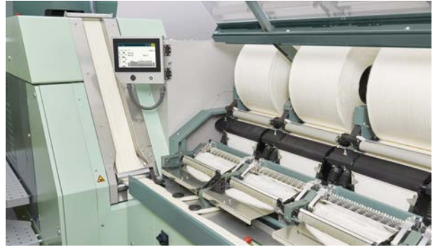
The new comber E 90 produces highest sliver quality thanks to the integrated SB-D 50 draw frame technology.
