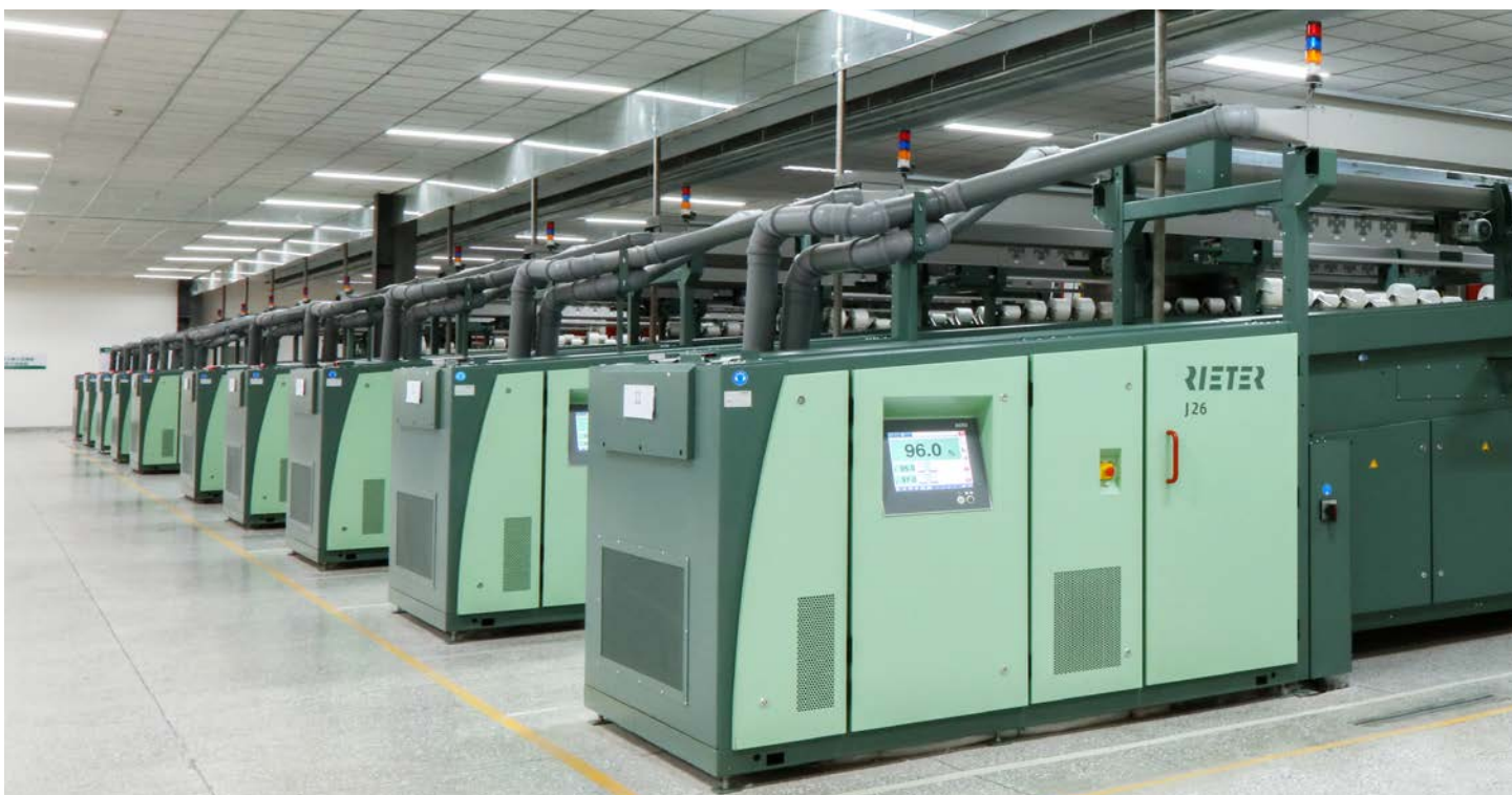
A Rieter spinning mill with the air-jet spinning machines J 26 produces unique cotton yarns extremely economically.
