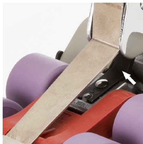
Fig. 3: top roller weighting unit with leaf spring
