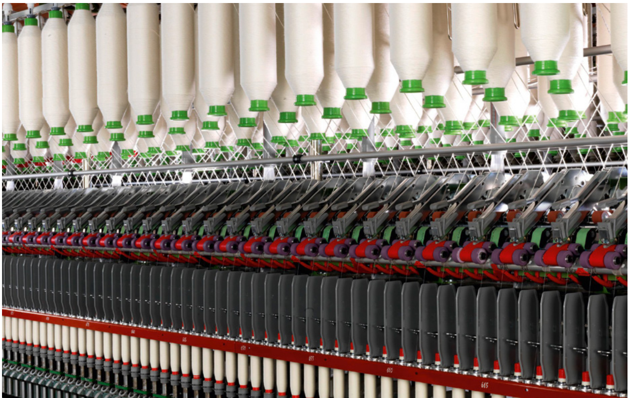
EliTe®Compact Spinning System on Hermann Bühler ring spinning machine
