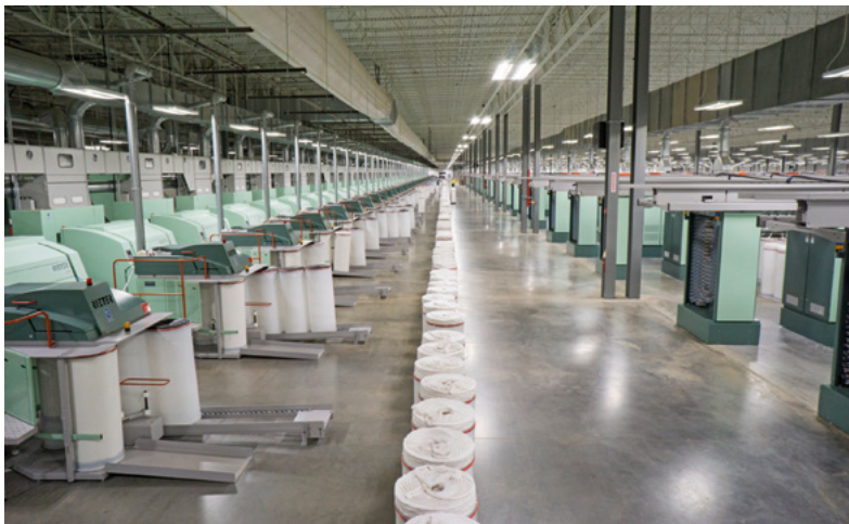
Gildan Salisbury's line up of Rieter C 70 cards and R60 spinning frames
