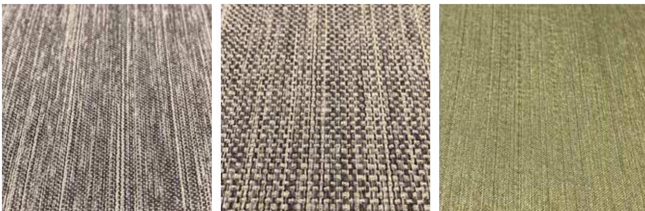
Used on a single-color thread, a rather subtle dullness modulation is produced; the fabric shows lengths with contrasting intensities of sheen
